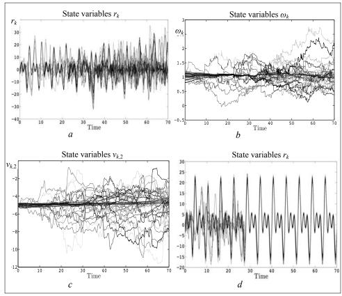
Fig. 4. Time evolution of  $r_k$  (Fig. 4,a),  $\omega_k$  (Fig. 4,b) and  $v_{k,2}$  (Fig. 4,d) for 39 PSS, interacting through the network in (Fig. 2,b). Time evolution of  $r_k$  for 39 PSS with all their adaptive mechanisms switched off (i.e. all susceptibility constants are zero), interacting through the network in (Fig. 2,d)
