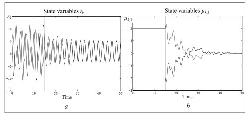
Fig. 5. Time evolution of  $r_k$  (Fig. 5,a) and  $\mu_{k,1}$  (Fig. 5,b) for two PSS. Coupling dynamics and adaptive mechanisms are switched on a t = 15 (black solid line).
