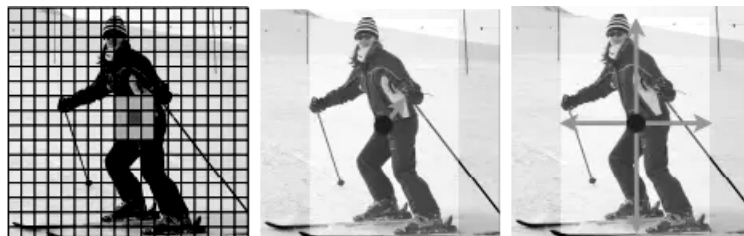
Fig. 4. Left: keypoint heatmap; middle: keypoint offsets; right: dimensions of box (source: original paper [10])
