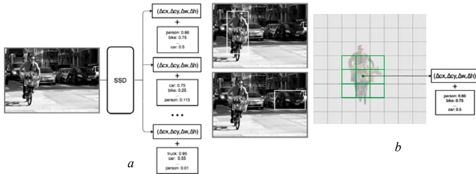
Fig. 19. Multibox predictor — a ; convolutional predictors for object detection (source: article — b [47])
