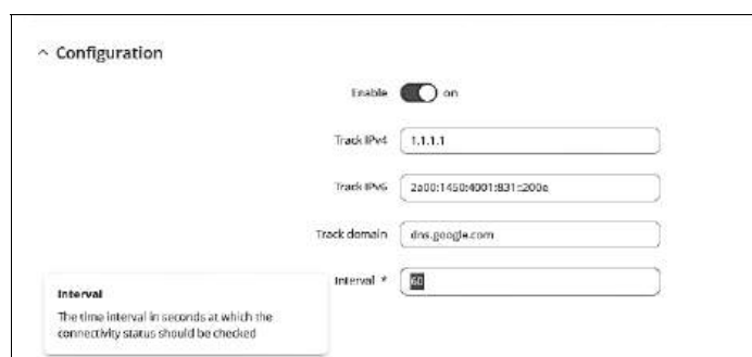
Fig. 2. Connection state polling interval parameter for RUT routers
